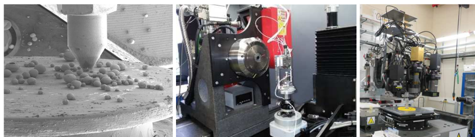
Fig 1 : (Left to right), Agglomerates forest on stub during micro-compression tests in SEM of Atalante facility, tomograph in Charles Sadron Institute, tomograph in Anatomix beam line synchrotron Soleil.
