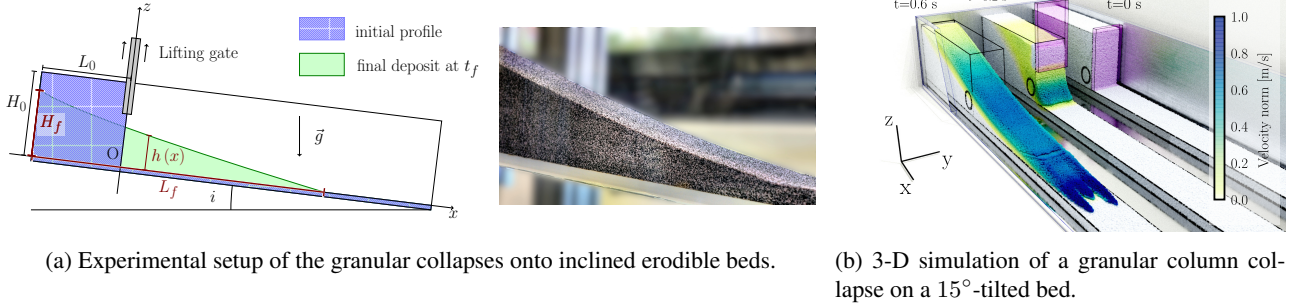
Figure 1. Inclined granular column collapses: experiments and simulations [1].
